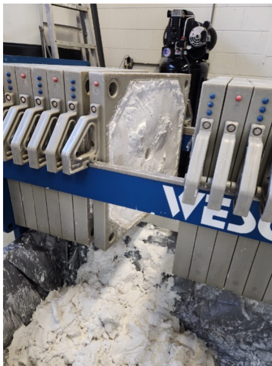
Image 2: Filter press used in the conversion process to produce lithium carbonate
