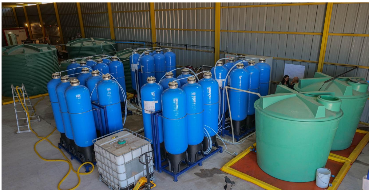
Figure 4: CTL's pilot plant at the Company's R&D Centre in Copaipó. The blue columns (approx. 2.5 metres tall x 30) are loaded with Lanshen's resin. The green bioplastic vessels on the right will feed the columns with brine from Laguna Verde.
